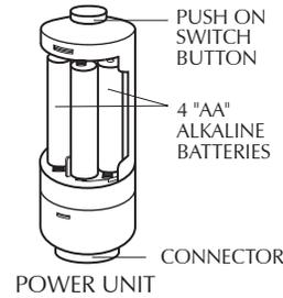
**NOTE: ALWAYS USE ALKALINE BATTERIES FOR THE BEST GRINDING EFFICACY**
